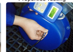
Coating Thickness Check
